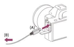
A: To the Multi/Micro USB TerminalB: To the USB jack of the computer
