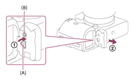
• You can attach the removed battery cover to the vertical grip so that you do not lose it.
