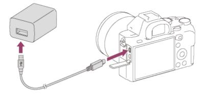
Charge lamp Lit: Charging Off: Charging finished Flashing: Charging error or charging paused temporarily because the camera is not within the proper temperature range
