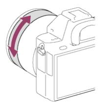
• When you rotate the focus ring, the focus distance is displayed on the screen.
